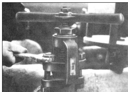
Step #2: Packing gland nuts are then removed, gland flange is lifted and split glands removed. Thread bushing and handwheel nut are loosened.
