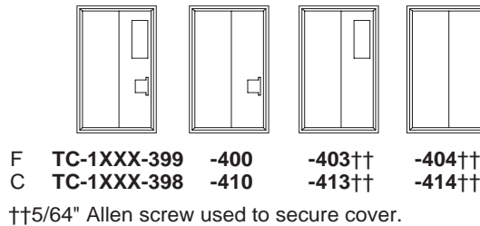
Figure 2 Options (for quantities of 24 or more each number) Add dash number (-XXX) suffix to base [part number of desired option]. For metal covers, specify TC2-11XX. No cover option for TC-1XX.
