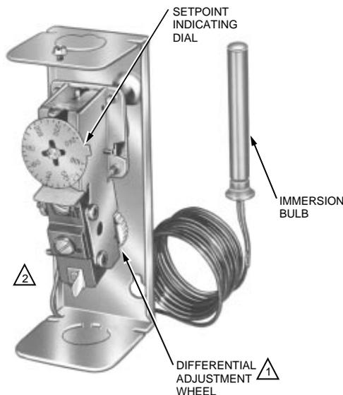
1 ONLY MODELS WITH ADJUSTABLE DIFFERENTIAL HAVE ADJUSTMENT WHEEL. STANDARD MODELS ARE FIXED AT APPROXIMATELY 5°F (3°C).
