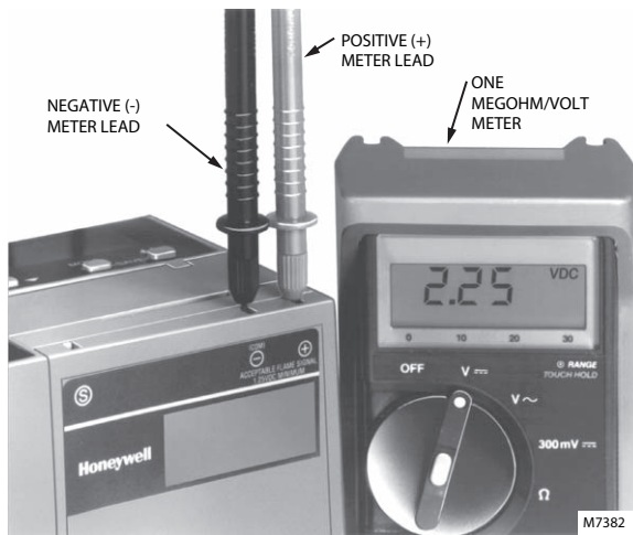
Fig. 11. Measuring flame signal voltage of 7800 SERIES controls.
