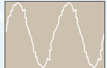
12-pulse input with phase-shift transformer.
