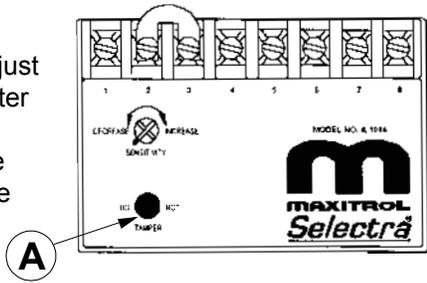
**If calibrating at the TD114 Remote Temperature Selector:** If measured temperature is below set temperature, rotate the calibration potentiometer clockwise until the correct temperature is obtained. If the temperature is above the set point the potentiometer should be turned counter-clockwise. Proceed slowly with the above steps so as to allow the temperature measuring instrument to catch up with the change in temperature.
