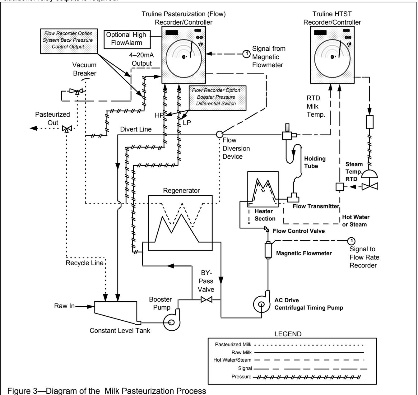
Figure 3—Diagram of the Milk Pasteurization Process
